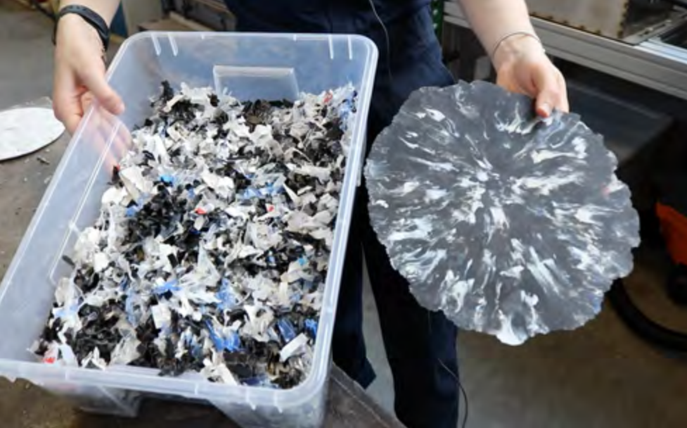
ABOVE: PLASTIC IS CLEANED AND SHREDDED BEFORE BEING FORMED INTO A SHEET OR BLOCK
