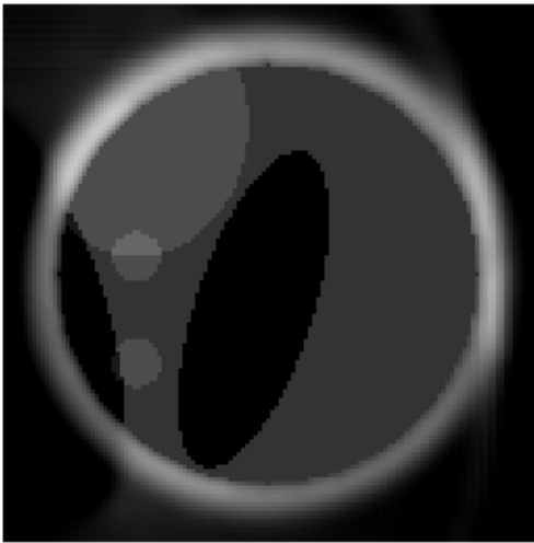
Figure 4.10: Reconstruction through Searchlight CT from the soft partial collimated X-ray Transform shown in Figure 4.9
