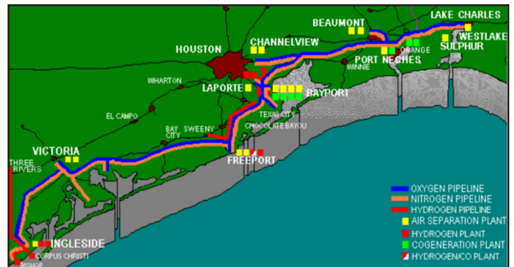
Figure 2: Air Liquide H 2 Pipelines (Air Liquide 2005).
